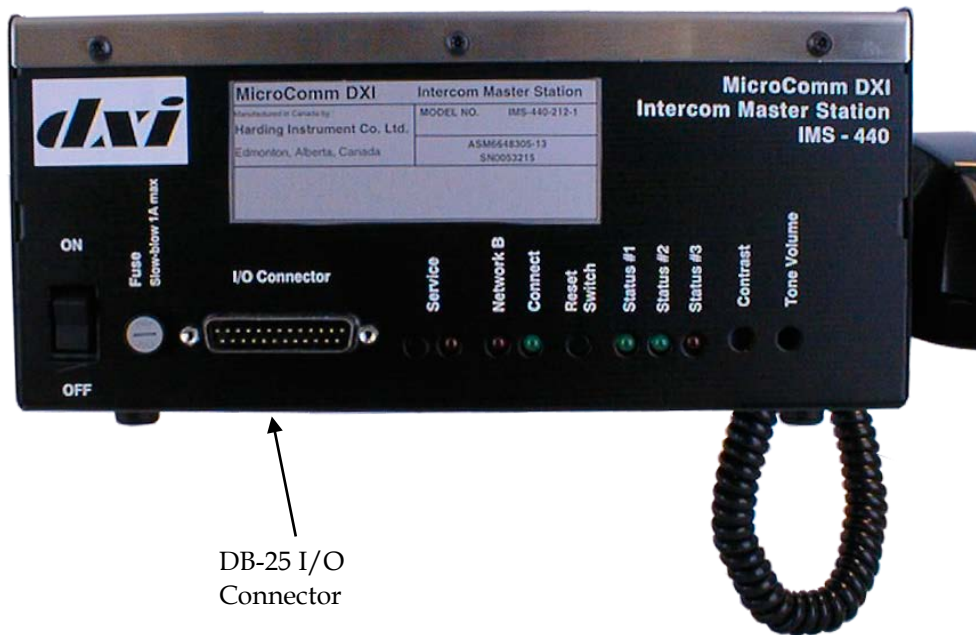
Back of IMS-440 Intercom Master Station Showing Location of DB-25 Connector
