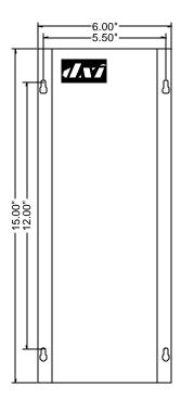
Mounting Hole Detail of PSU-123 (PSU-125) power supply
